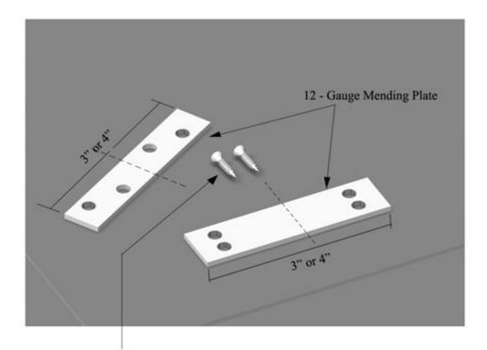
3/4"Long #12 Screw or 1/4" Dia Bolt with 2" Dia Washer and Bolt.
