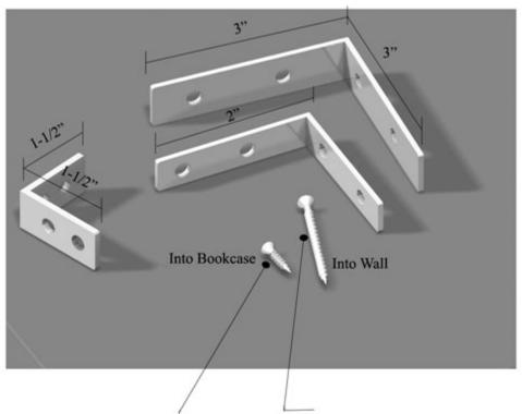
3/4"Long #12 Screw or 1/4" Dia Bolt with 2" Dia Washer and Bolt. #12 Wood Screws (for Wood Studs):
