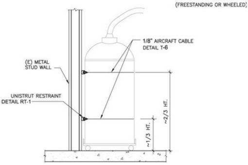
Universal Tank Restraint (Metal Stud Wall)
