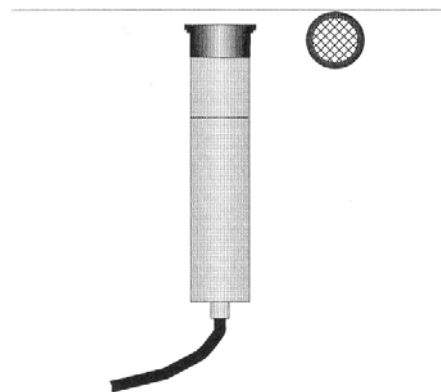
Figure 6. Victoreen 489-35 end-window G-M detector
