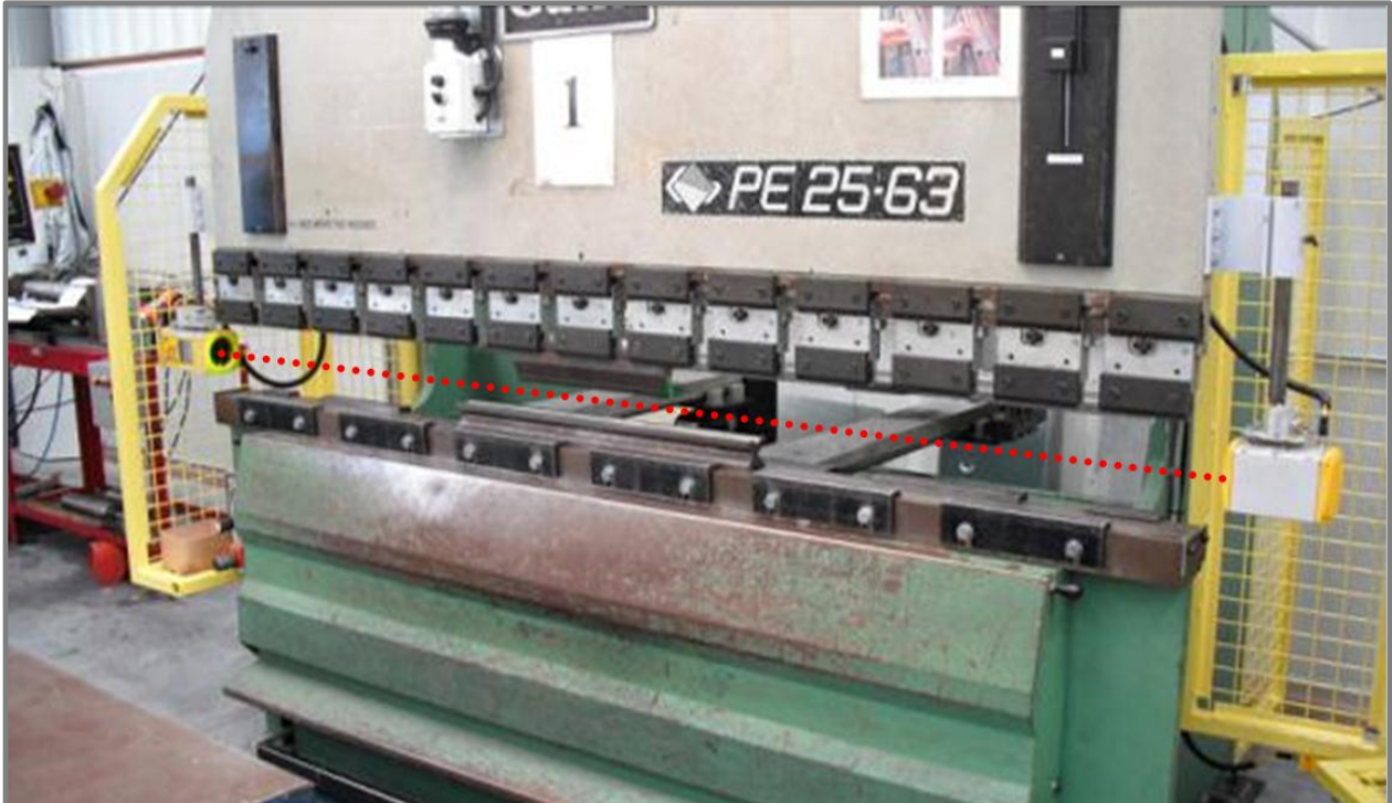
Optical light beam on a press.
