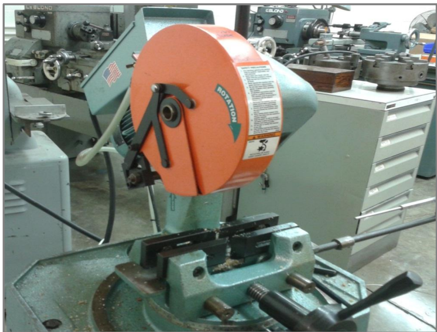
Chop Saw with Self-adjusting Guard
